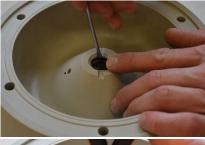
**Fig. 3.6.1**Using a screwdriver, insert the O-rings [47] into the dampener block [12].
