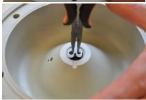
**Fig. 3.6.2**Using a pair of pliers, insert the seals
