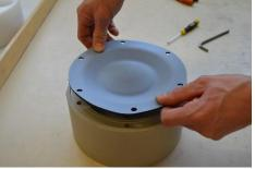
**Fig 3.5.6** Unscrew the diaphragm [15] by hand (clockwise).
