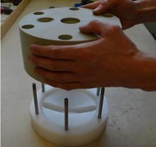
**Fig. 3.5.4**Take out the dampener block [12].
