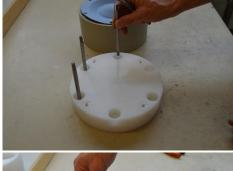
**Fig. 3.5.5**Take the pin screws [14] out of the dampener housing [11].
