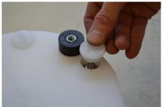
**Fig. 3.5.2** Remove the nut covers [579] from the dampener housing and block
