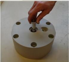
**Fig 3.5.8**Push out the shaft [1651] from the dampener housing
