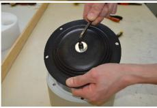
**Fig 3.5.7**Using an allen key, unscrew the shaft ending [1652] from the diaphragm.
