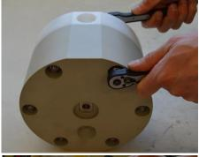
**Fig. 3.5.3**Using two spanners unscrew the nuts [37] cross-side and take them out alongside with the washers [38].
